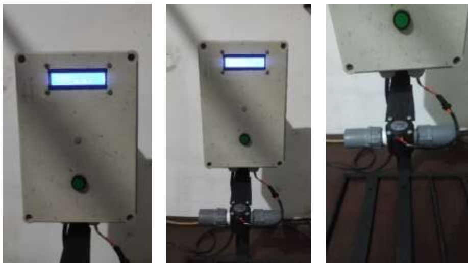
Figure 4. Device Recording of Wastewater Outlet Water Discharge from IPAL
