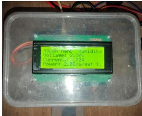
Figure 7. I2C 20x4 LCD Display.
