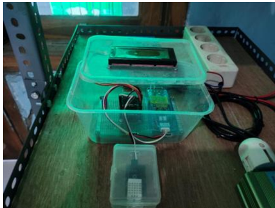
Figure 5. DHT 22 Sensor Testing Process.
