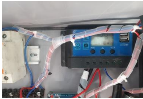
Figure 4. Process of Testing Solar Panel Charging When Displayed on SCC.
