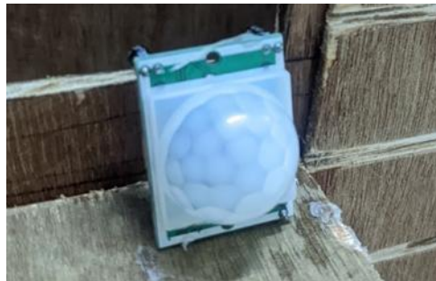
Figure 5. View of the PIR Sensor Installed on the Device.
