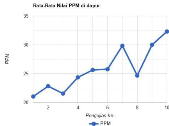
Figure 6. Graph of PPM Value for medium fan speed.
