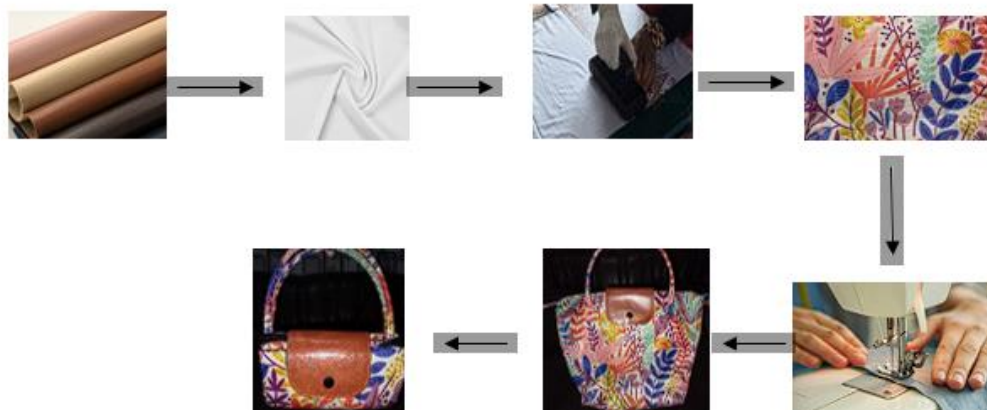
Figure 2. A Simple Overview of the Design Development Manufacturing Flow Using the Atumics Method in Leather Bag Products
